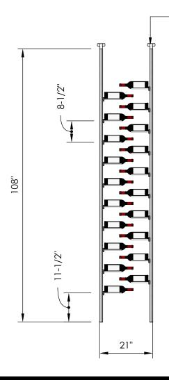
Telescopic bracket allows height to be extended up to 112"
