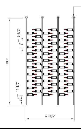
Telescopic bracket allows height to be extended up to 112"
