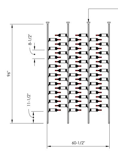
Telescopic bracket allows height to be extended up to 100"
