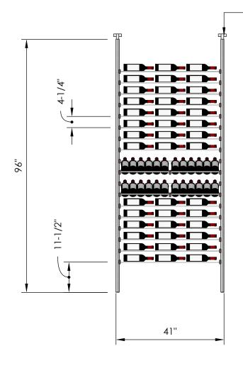
Telescopic bracket allows height to be extended up to 100"
