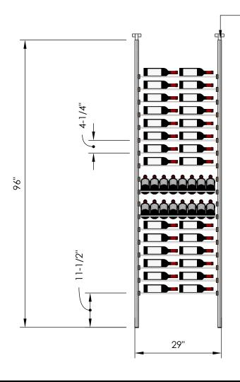
→ Telescopic bracket allows height to be extended up to 100" (Post can be cut down by up to 4 inches for a racking height as low as 92")
