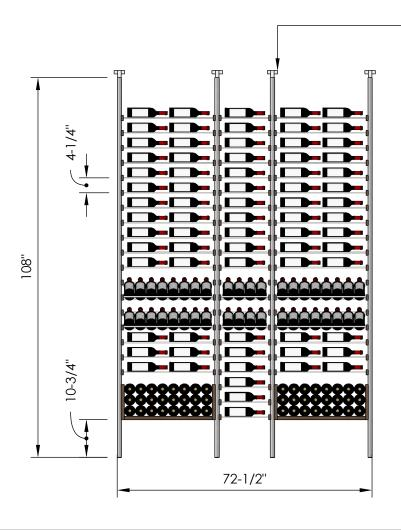
Telescopic bracket allows height to be extended up to 112"
