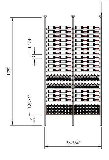
Telescopic bracket allows height to be extended up to 112"
