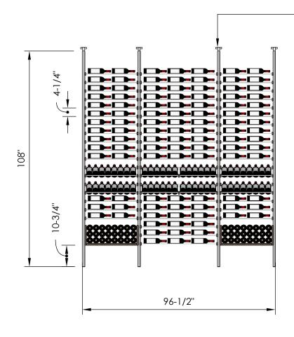
Telescopic bracket allows height to be extended up to 112"
