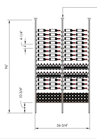
Telescopic bracket allows height to be extended up to 100"
