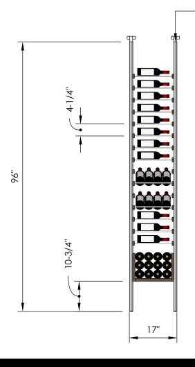
→ Telescopic bracket allows height to be extended up to 100" (Post can be cut down by up to 4 inches for a racking height as low as 92")
