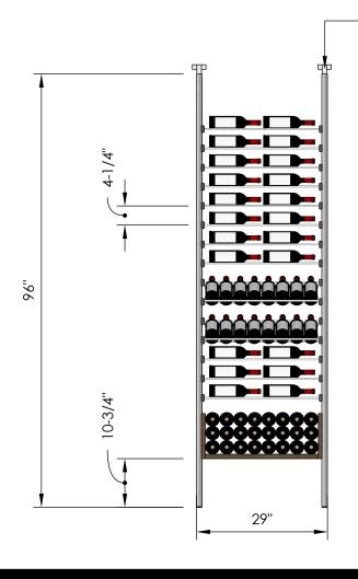
Telescopic bracket allows height to be extended up to 100"
