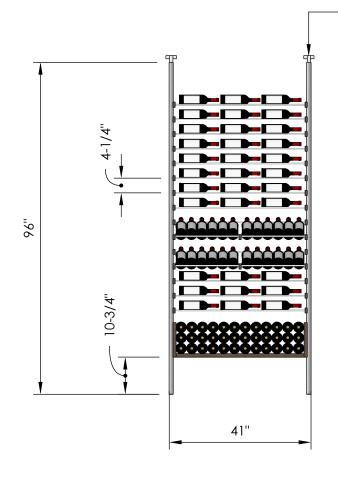
→ Telescopic bracket allows height to be extended up to 100" (Post can be cut down by up to 4 inches for a racking height as low as 92")
