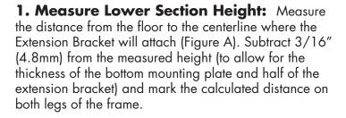
**Note:** If the calculated measurement aligns with one of the cross members, cut 2" (52mm) off the end of the frame and then mark the cut lines, measuring away from the fresh cut.
