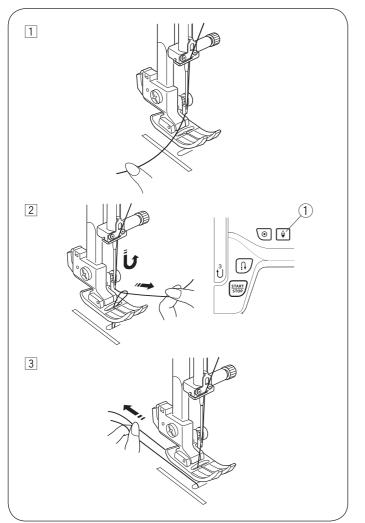
**Drawing up the Bobbin Thread** Raise the presser foot. Hold the needle thread lightly with your left hand.
