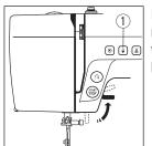
Raise the presser foot. Press the needle up/down button ① to raise the thread take-up lever to its highest position.
