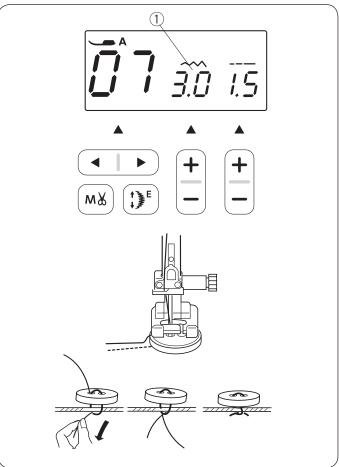
Lower the feed dog (refer to page 16). Set the speed control slider at a slower speed.
