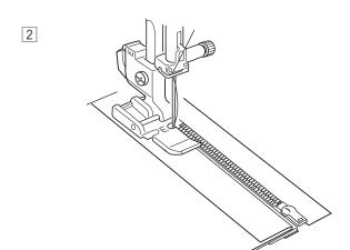
2 Attach the zipper foot E with the pin on the right hand
