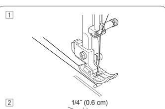
1 Loosen the thread tension to "1" and increase the stitch length to 5.0.
