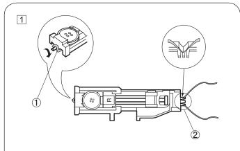
1 Use the same procedure as the standard buttonhole sewing. Set the stitch width to match the thickness of the cord used.
