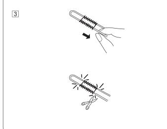
3 Pull the loose ends of the filler cord to tighten it.
