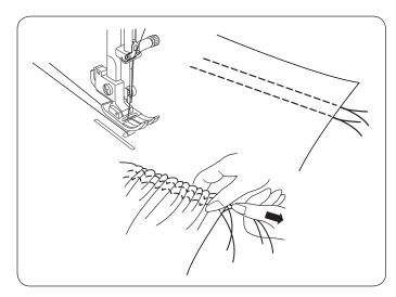
Loosen the thread tension to "1" and increase the stitch length to 5.0.
