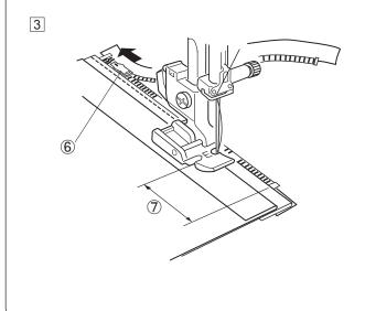
3 Sew through all layers next to the fold. Stop the machine 2" (5 cm) before the foot reaches the slider on the zipper tape.
