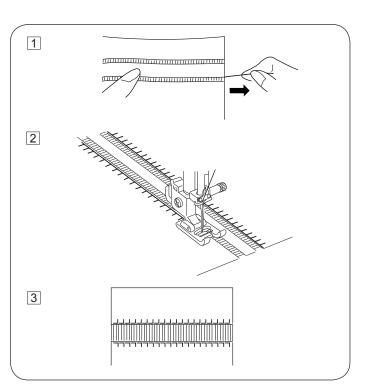
Drawn work uses the same method as fringing. Choose a firm, woven fabric like linen where threads can be removed easily.
