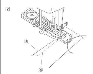
2 Start the machine and sew the buttonhole. Each side of the buttonhole and the bartacks will be sewn over the cord.
