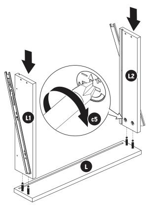
Attach Panels L1 and L2 to Panel L as shown above. Tighten cams and apply **c2 Cam Covers.** Repeat with remaining 6 drawers (7 total).
