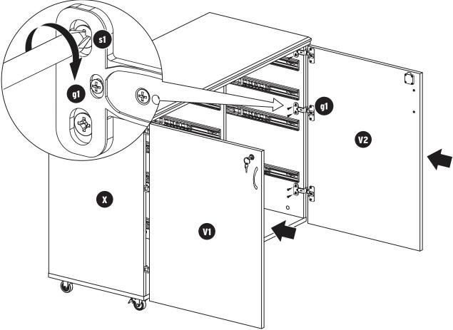
Attach g1 Hinge Body on Panels V1 and V2 to Panels X and Z with s1 Screws.
