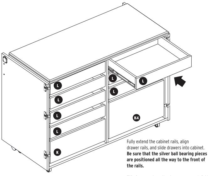
**TIP:** Once you hear the drawer runners "click" into place, gently open and close the drawers a few times to engage the Soft Close mechanism.
