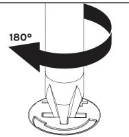
Screw cam bolts flush as illustrated.
