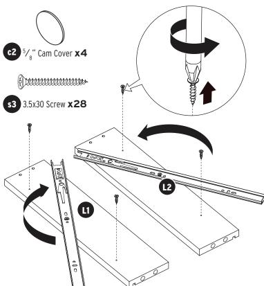
To reach the pre-drilled screw holes on the sides of Panels L1 and L2, you will need to tilt the drawer runners.
