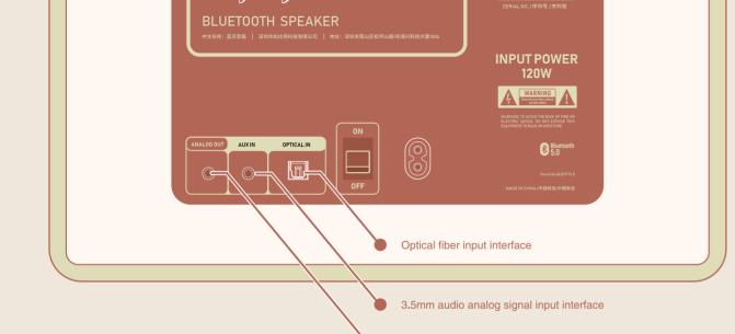
Analog output interface: When the speaker needs to be used as an output source signal, a 3.5mm audio cable is connected to the "ANALOG OUT" interface to synchronize the sound source of the speaker.
