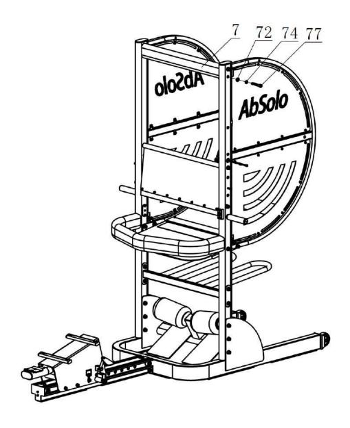
1. Attach the Target (#41) to the Uprights ASSY with Upper Tube (#11) using: two Φ26\*Φ20\*59 Upper Spacer (#31)
