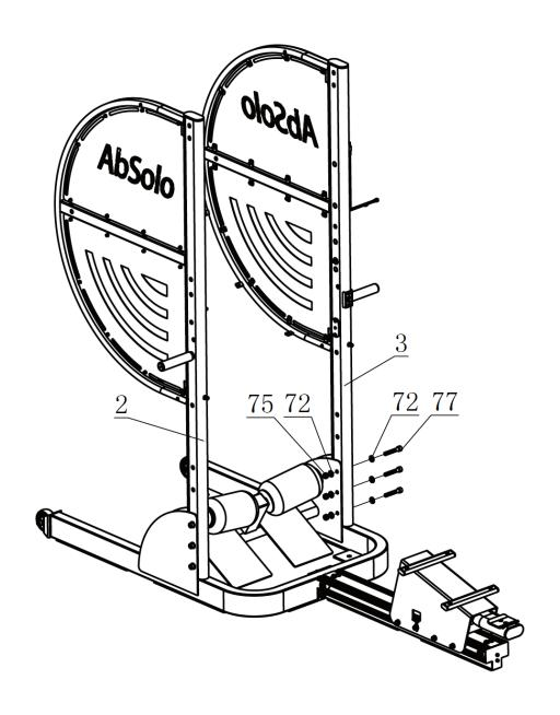
1. Attach Ball Rack (#4) to the both sides of the Uprights using: two Reinforcement Plates (#20) four M10\*60 Socket Head Cap Bolts (#77) eight Φ11\*Φ20\*2 Flat Washers (#72) four M10 Nylon Lock Nuts (#75)
