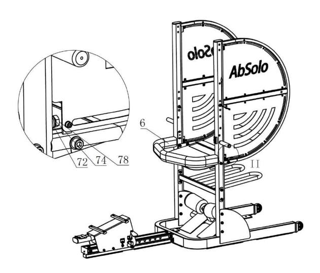
1. Attach Bull's Eyes Baffle (#8) to the Uprights ASSY using: four M10\*60 Socket Head Cap Bolts (#77) four Φ10 Spring Washers (#74) four Φ11\*Φ20\*2 Flat Washers (#72)
