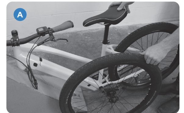
(A) Remove the front wheel from the left side of the bike, and remove the plastic hub protectors from the ends of the wheel hub.
