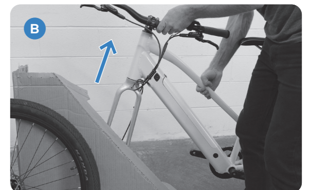
(B) Remove bike from triangle holder, lifting by the handlebars and frame.
