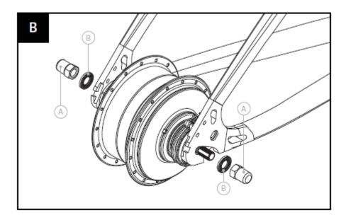
Note that the non-turn washers have a "key" which slots into the horizontal dropout on your Vvolt.
