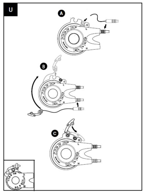
Install the Underdrive cable end (small end) into the forward cable end slot on the hub interface, then install the Underdrive cable housing into the top housing stop.
