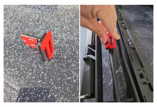
To ensure that the lettering sits in the middle and the spacing of the letters matches each other, please keep a distance of **12.5 cm** from the left edge of the grill to the first letter and glue the letters to each other at a distance of **1 cm**. Before you remove the 3M protective tape, it is recommended to try it out!
