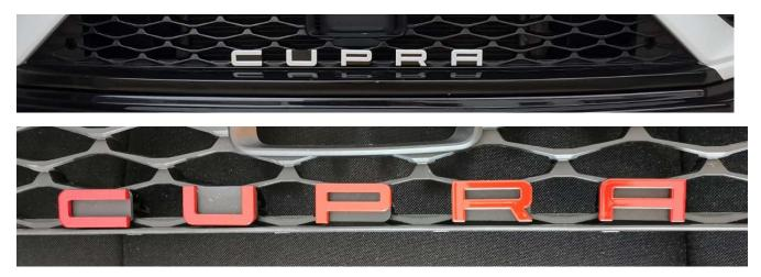
2. For vehicles without ACC, the lettering can also be clicked above, but **ALWAYS** only the place where the vertical honeycomb strut is:
