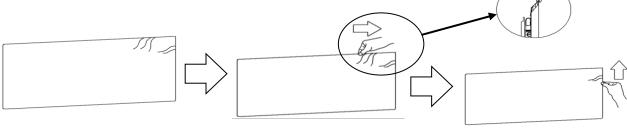
**Incorrect material installation** —The corners of the screen material are not properly wrapped along the edge of the frame leaving the material with unbalanced tension and an uneven finish. To correct, detach springs from material at the corner(s) where material does not lie flat along the edge of the frame, reposition the material so that it lies flat and wraps along the edge of the frame, and reattach springs to the material.
