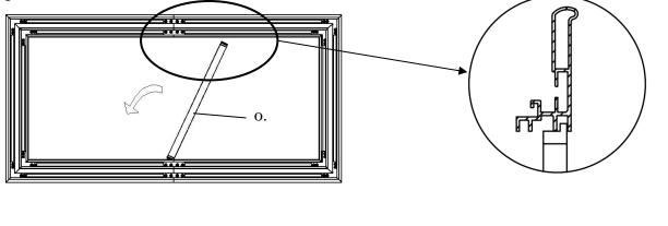
**Step 8:** Hook one end of the spring and secure inside the groove of the frame, use the *spring hook* (*h*) to attach the spring to the hole located on the screen material's outer edge in the following order.
