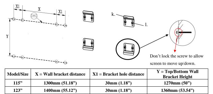
**Step 14**: Position the fixed frame screen onto the bottom brackets (fig 1) as shown below and push down at the center of the top of the frame on the top bracket (fig 2) to secure the frame installation.
