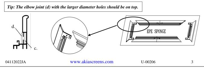
Step 5: Secure the elbow joints by fastening them with M4x7 screws (g), 4 at each corner.
