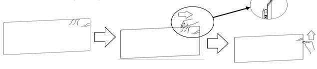
**Incorrect material installation** –The corners of the screen material are not properly wrapped along the edge of the frame leaving the material with unbalanced tension and an uneven finish. To correct, detach springs from material at the corner(s) where material does not lie flat along the edge of the frame, reposition the material so that it lies flat and wraps along the edge of the frame, and reattach springs to the material.
