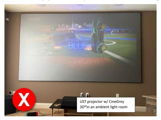
Image shows how a UST projector with CineGrey 3D® looks like in a room with lights turned off. The image appears to look good butis still reflecting the projector light upwards and causing a hotspot in the middle of the image.
