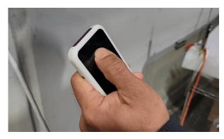
**Step 3.** While holding the UP button, plug the screen back to the power outlet. (The screen should drop and retract to confirm the sync process)
