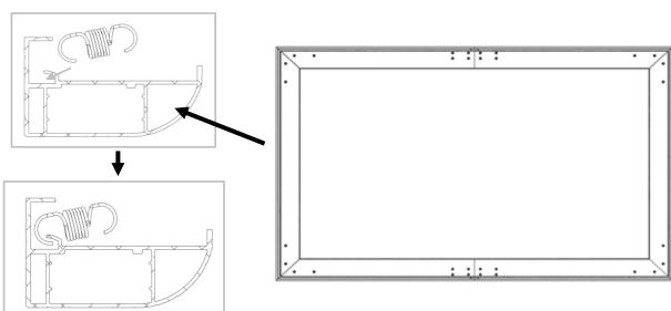
**Step 8.** With one end of *the Spring (B)* hooked on the back of the frame, hook the end of the *Spring* through the hole located on the screen material's outer edge. **Be sure to hook the** *Springs (B)* **onto the** *Tension Rod (I)* **to avoid damage to the screen material.** Use the *Pull Hook (E)* when necessary. Attach the four corners and center horizontal sections of the material (1).
