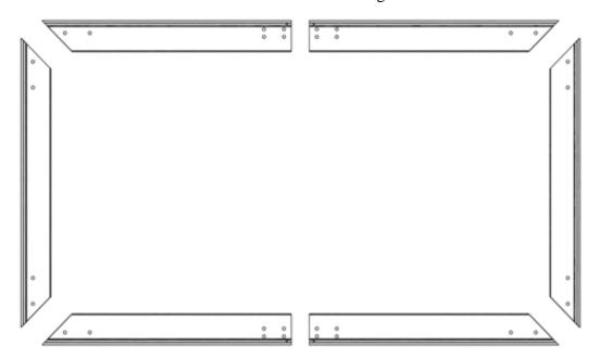
**Step 3.** Insert the *Center Joint* (A) connector into one-half of the Horizontal Frame (B) and fasten with two Large Screws and Washers (D). Once secure, connect with the one-half of the Horizontal Frame (C) and fasten with two Large Screws and Washers (D). Repeat steps for the other one-half of Horizontal Frames (B) and (C).
