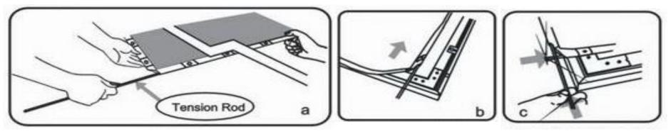
**Step 7.** Hook the *Springs* (*B*) on the back of the frame. Line them up with the corresponding holes on the materials edge. Be sure the hook is secure and hook the other end to the corresponding hole on the material. For the correct amount of springs to place on the frame/material, please refer to the table listed below.
