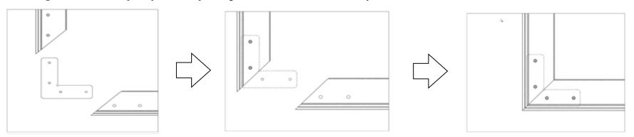
Note: You may have to loosen and adjust the brackets and frame pieces. It will help to leave the screws loose until perfect right angles are formed, then tighten the screws securely.
