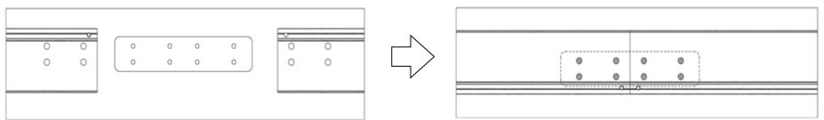
**Step 4.** Insert the *Elbow Joints* (*C*) to top and bottom sections of the *Vertical Frame* (*A*). Once inserted, secure the *Elbow Joints* (*C*) by fastening them with the *Large Screws and Washers* (*D*) and connect the *Vertical Frame* sections to the *Horizontal Frame* sections. Make sure all corner frame pieces are flush (no gaps). They should form perfect right angles.
