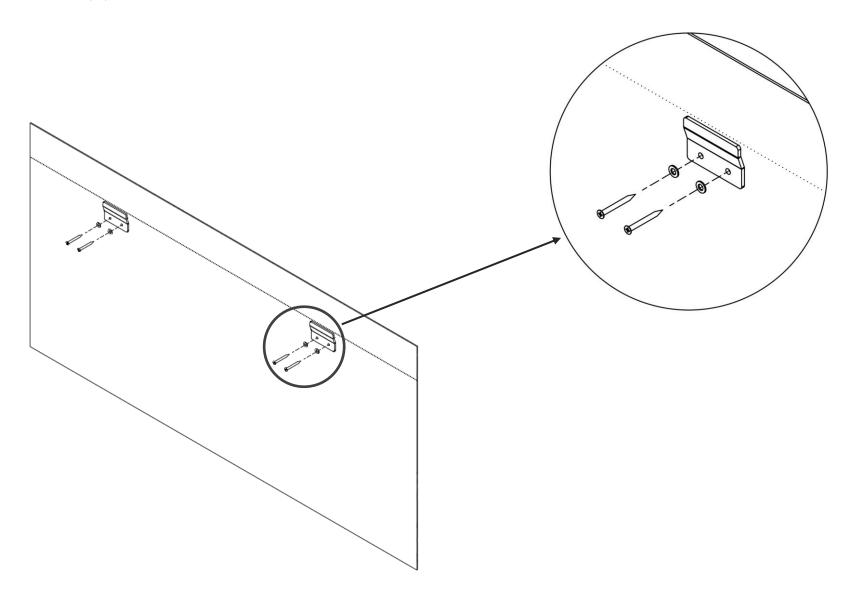
**Step 12.** Position the Fixed Frame Screen onto the wall *Brackets* (*F*) as shown below and push down at the center of the top of the Frame to secure.
