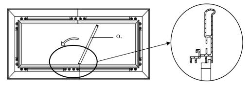
**Step 10:** Hook one end of the spring and secure inside the groove of the frame, use the *spring hook* (*h*) to attach the spring to the hole located on the screen material's outer edge in the following order.
