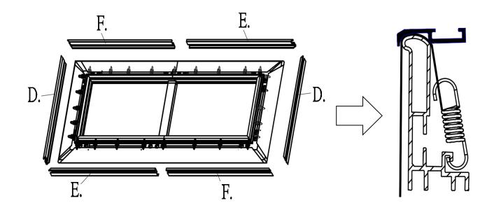
Connect edge trim frames (e/f) together using the M4 center joint (e) and secure with four of the M4x4 screws (m) as show in Step 1. Repeat for other side.
