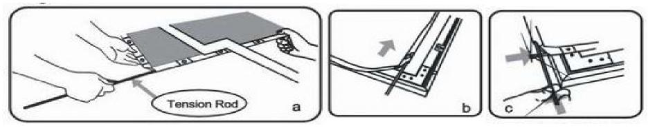
**Step 7.** Insert the *Springs (B)* into the grooves of the frame. Line them up with the corresponding holes in the materials edge. Be sure the shorter hook on each spring is placed in the frame's groove, while the longer hook attaches to the material. For the correct amount of springs to place into the frame, please refer to the table listed below.
