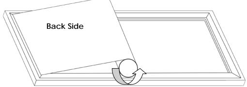
**Step 6.** Insert the four horizontal and two vertical *Tension Rods (I)* into the corresponding sides of the screen material, while keeping the material laying flat. Careful not to snag on the holes at the edge of the material during this process; forcing the rods may damage the screen material.
