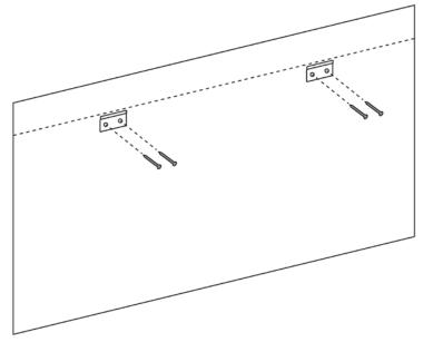
Step 12. Position the fixed frame screen onto the wall Brackets (F) as shown below and push down at the center of the top of the frame to secure.
