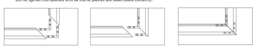
Note: You may have to loosen and adjust the brackets and frame pieces. It will help to leave the screws loose until perfect right angles are formed, then tighten the screws securely.
