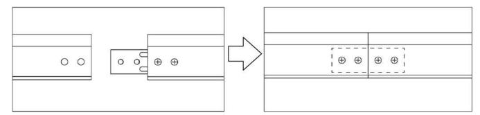
**Step 4.** Insert the Elbow Joints (C) to top and bottom sections of the vertical frame. Once inserted, secure the Elbow Joints (C) by fastening them with the Small Hex Screws (D) and connect the vertical sections to the horizontal frame sections. Make sure all corner frames pieces are flush (no gaps). They should form perfect right angles.
