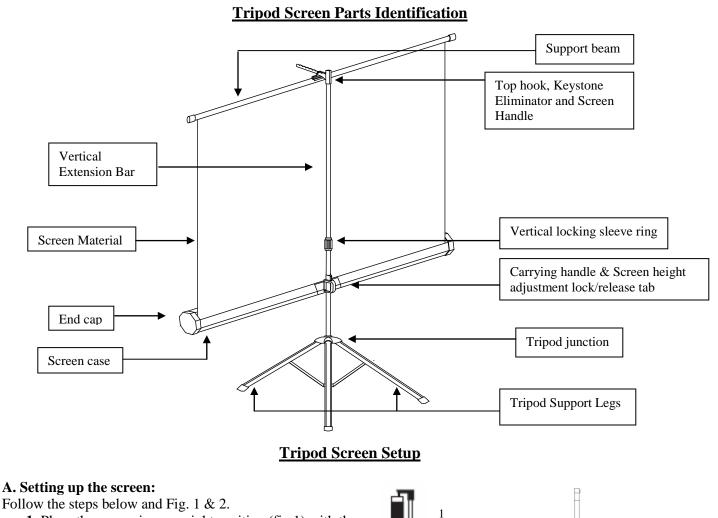
**1.** Place the screen in an upright position (fig.1) with the legs toward the ground.
