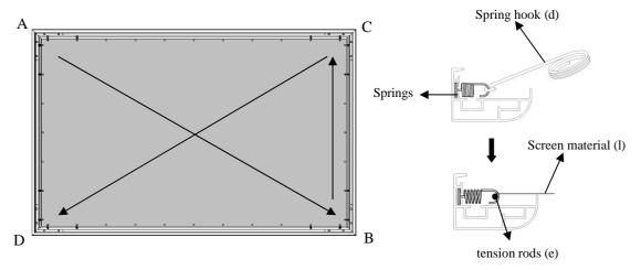
5. Install all the spring on screen material, install the spring at position 1, then continue to install the spring at position 2, then finally install the rest of spring on the screen material, shown as below.
