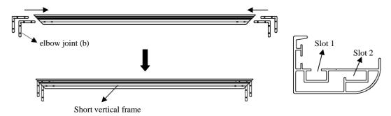
4. Then insert the horizontal long frames into the exposed *elbow joint* (*b*) connectors and fasten them with M5\*6 screws (c).
