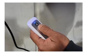
**Step 3.** While holding the STOP button, plug the screen back to the power outlet. (The screen should drop and retract **TWICE** to confirm the sync process)
