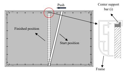
This will provide added stability to your frame and added tension to the material.
