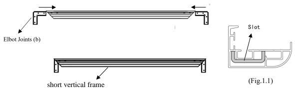
4. Insert the long frame into the exposed *Elbow Joints* (b) connectors and fasten them with M5\*6 screws (c) (Fig.1.2).
