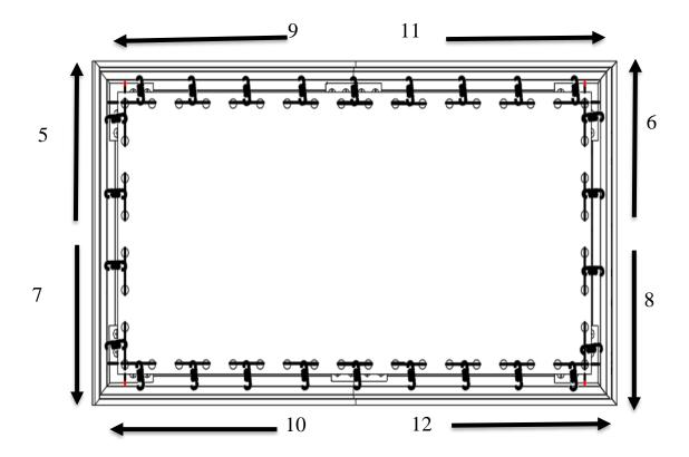
**Step 10**: Insert the Center Support Bar (o) into the upper top groove on the back of the frame with the bottom end near the approximate center point of the frame and rotate it in at an angle so that both ends of the bar are in alignment with the groove.
