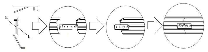
**Step 4:** Connect the *elbow joints (c/d)* to the top and bottom sections of the vertical frame. Once inserted, connect the vertical sections to the horizontal frame sections. Make sure all holes are in alignment and the frame pieces are flush (no gaps). They should form perfect right angles.
