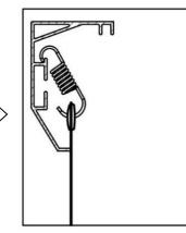
First connect on four corners, steps 1-4. make sure all four corners are fixed before proceeding with next spring.
