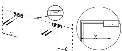
wood screws with a screwdriver. Make sure the brackets are leveled.
