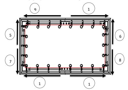
**Step 9**: Insert the Center Support Bar (o) into the upper top groove on the back of the frame with the bottom end near the approximate center point of the frame and rotate it in at an angle so that both ends of the bar are in alignment with the groove.
