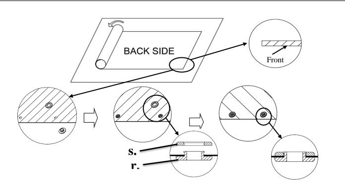
**Step7**: Carefully place the screen on top of the assembled frame as shown below. Make sure that the angular **edges** of the frame are not allowed to come into direct contact with the screen material to avoid puncturing.
