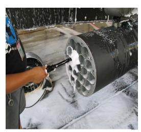
Foaming brush applicator that is applying 725 Cleaner/Degreaser to a rocket pod.
