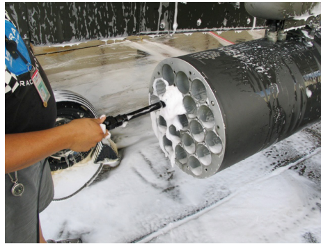
Foaming brush applicator that is applying 725 Cleaner/Degreaser to a rocket pod
