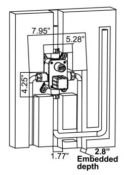
5. Drive the rubber plug into the wall, and fix the main body to the wall with screws.
