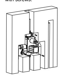
6. After the faucet is connected to the water pipe, test the water normally, keep the pressure for one minute, and check whether there is any water leakage.
