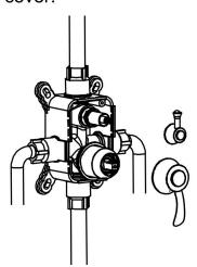
8. Remember to put the protective cover back on before tiling the tiles, and tighten the screws to prevent the surface of the valve body from being damaged.
