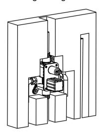
9. After the tile is applied, remove the protective cover, cover the decorative panel, and install the handle and handwheel.
