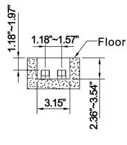
4. Connect the inlet tube like the drawing.
