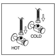
5. Attach flexible hose to water supply.
