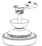
Slide the receiver into the open end of the mounting bracket with the flat side of the receiver facing the ceiling.
