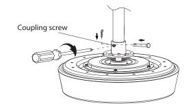
Slide downrod into the coupling on top of the motor. Install the hanging pin by aligning the holes in the coupling with holes in the downrod. Secure hanging pin with locking pin. Securely tighten the two previously loosed set screws.
