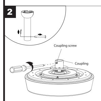
Loosen the two coupling screws preassembled in the coupling, but do not remove them. Remove the locking pin and hanging pin from the downrod assembly. Retain for later use.
