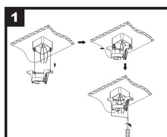
Screw the two mounting screws and washers to the outlet box. Slide the mounting bracket onto the screw through the T-slot.
