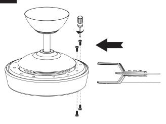
Position blade assembly along the motor and make sure the blade arm is fully seated against the flywheel. Tighten them with four blade screws.
