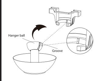
Carefully lift the fan and seat the downrod/hanger ball assembly onto the mounting bracket that was just attached to the outlet box. Be sure the groove in the ball is lined up with tab on the mounting bracket.
