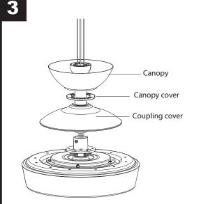
Place downrod assembly through canopy, canopy cover and coupling cover. Route the motor lead wires through the downrod assembly.
