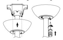
Loosen the screws without fully removing it. Assemble canopy by rotating key slot in canopy over screws in mounting bracket, taking care notto pinch the wires.
