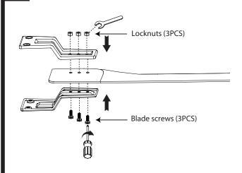
Attach blade arms to blade as shown. Screw the blade screws (provided in the hardware bag) into the screw holes and tighten it with the locknuts by using a wrench.
