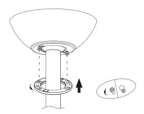
Securely attach and tighten the canopy cover over the screws in the mounting bracket utilizing the key slot twist-lock feature.
