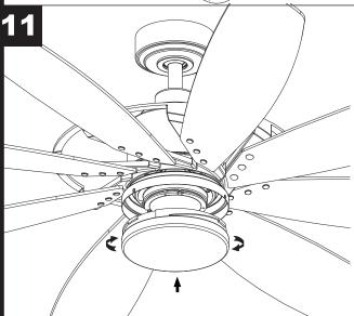
Secure the shade to the switch housing assembly by twisting in a clockwise direction.
