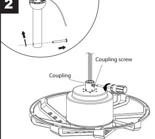
Loosen the two coupling screws preassembled in the coupling, but do not remove them. Remove the locking pin and hanging pin from the downrod assembly. Retain for later use.
