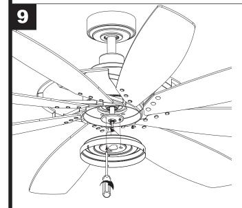
Assemble the switch housing to the support bracket using the two key slots. Replace the previously removed screw and securely tighten all three screws.
