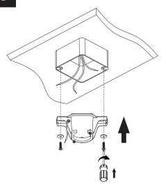
Securely attach the hanger bracket to the outlet box using the screws and washers provided in the hardware bag.
