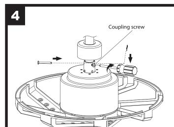
Slide downrod into the coupling on top of the motor. Install the hanging pin by aligning the holes in the coupling with holes in the downrod. Secure hanging pin with locking pin. Securely tighten the two previously loosed set screws.
