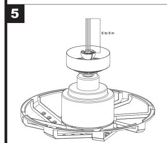
Cut off excess lead wire approximately 6 to 9 inches above top of the downrod. Strip insulation off 1/2 inch from the end of each lead wire.
