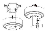
Loosen the screws without fully removing it.
