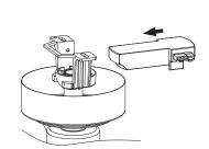
Slide the receiver into the open end of the mounting bracket with the flat side of the receiver facing the ceiling.
