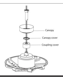
Place downrod assembly through canopy, canopy cover and coupling cover. Route the motor lead wires through the downrod assembly.
