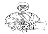
Remove one of the three screws in the support bracket at the bottom of the motor assembly and retain the screw for later and slightly loosen the remaining two screws.
