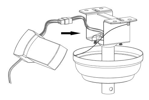
1.Carefully push the canopy to the bottom of the mounting bracket, make two sliding holes aligned to the two prominent screws on the mounting bracket, and then turn clockwise until tight.
