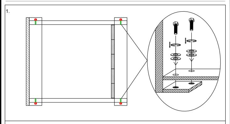
**Note:** Place the upper and lower tabletops vertically on a flat surface, and then thread the table legs from the lower tabletop into the upper tabletop. Align the hole positions of the table legs with the inner teeth of the upper and lower tabletops. Place the gasket on top of the hole position and screw in the mechanical screw. Tighten the mechanical screws in sequence from the top to bottom corners. Then use a wrench to tighten the mechanical screws in sequence.
