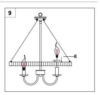
10. To adjust the length of the steel wire, gently press down on the wire clamp under the circular iron box. The other hand supports the steel wire that you want to adjust in length, inserting it inward to shorten it, and pulling it outward to lengthen it. When adjusting, always press and hold the wire clamp, adjust the length to a satisfactory level before releasing it.
