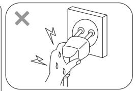
★ Wet hand is prohibited fror pulling or inserting power plug
