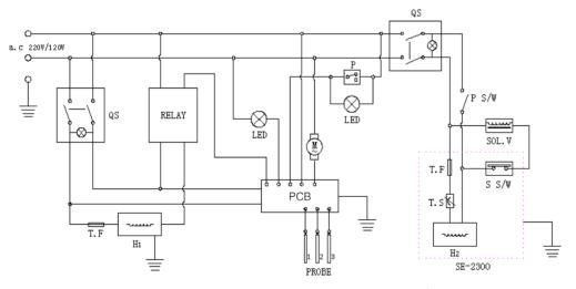
QS: power switch PCB: Pcb board
