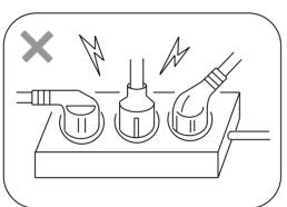
★ It must be used on the plue more than 120V/25A, 220V/15A individually.
