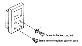
3 Oil shield plate assembly (THREE BOND TB 1104) Apply the sealant to the inside of the oil shield plate.
