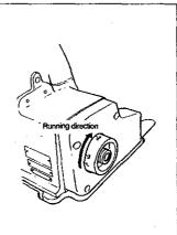
The correct machine running direction is such that the handwheel turns clockwise as viewed from the handwheel's side. Never run the machine in the reverse direction.
