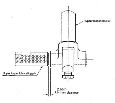
When the upper looper lubricating pin is set in place with the oil inlet faced upward, the lubricating hole is in the lower section as observed from this side.
