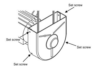
2-6. If necessary, adjust the position of the "protective rod" and "belt slip off prevention part mounting plate". Securely tighten after adjusting.
