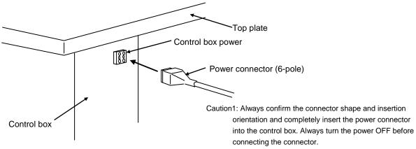
Caution2: Please do not bundle the power cable and other cables together. It may cause of malfunction by the influence of the power supply noise etc.
