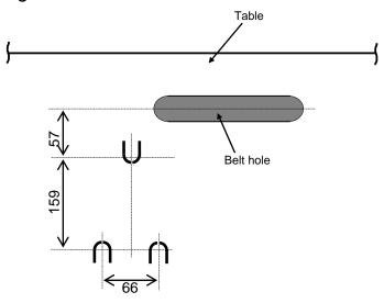
Correctly install the motor using the installation bolts, washers, spring washers and nuts.
