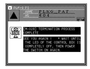
► After check the LED lamp on the front panel of the control box Is completely off, turn the power on.
