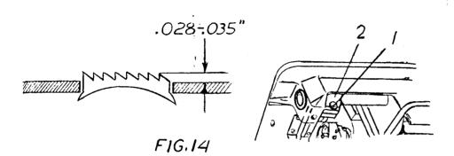
to obtain the desired rise of the feed dog. Be sure to tighten clamp screw (1) after the adjustment has been completed.
