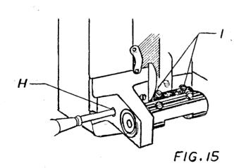
(Fig. 15) of the eccentric feed bar spindle. Enter a screw driver through hole "H" and turn the eccentric feed bar spindle slowly until the correct levelling has been reached. Tighten set screw upon completion of the adjustment.
