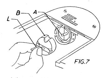
bobbin case and bobbin from rotary hook. While the latch is held open, the bobbin will be retained in the bobbin case. Release of the latch and turning of the open side of the bobbin case downward will cause the bobbin to drop out.
