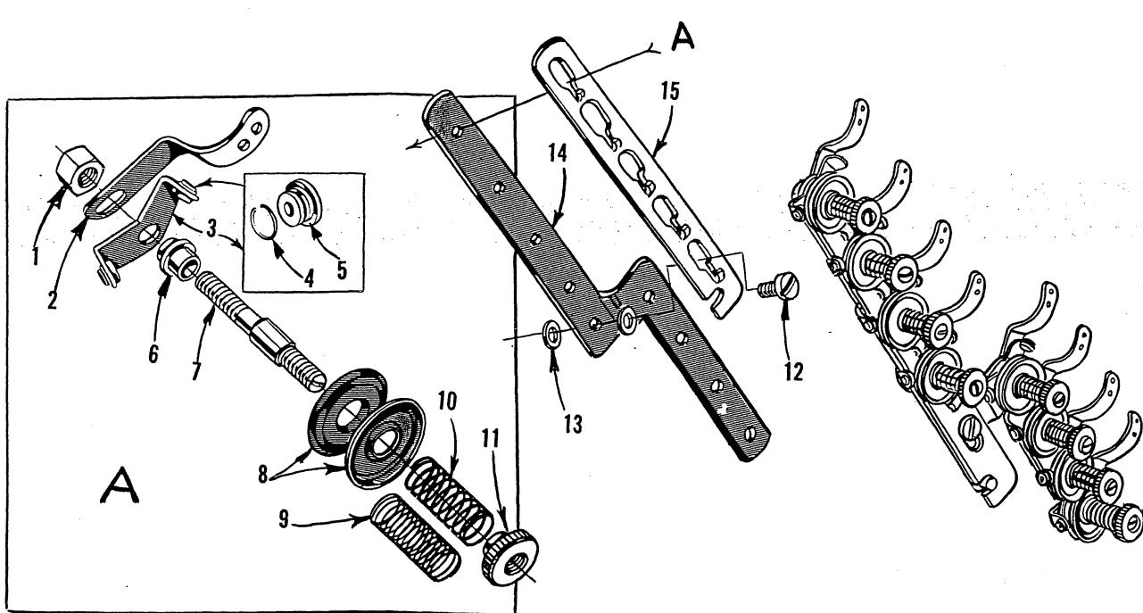
THREAD TENSION AND LIFTER LEVER PARTS
