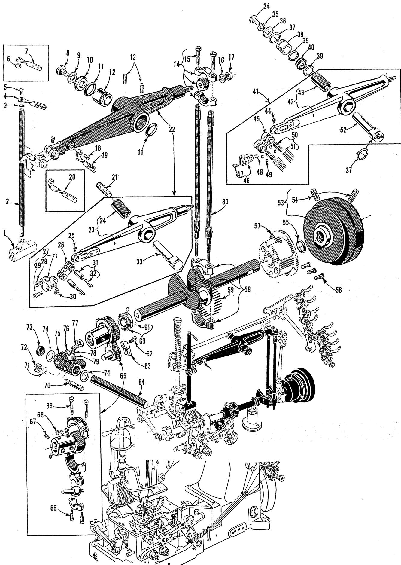
CRANKSHAFT, NEEDLE LEVER AND LOOPER DRIVING PARTS
