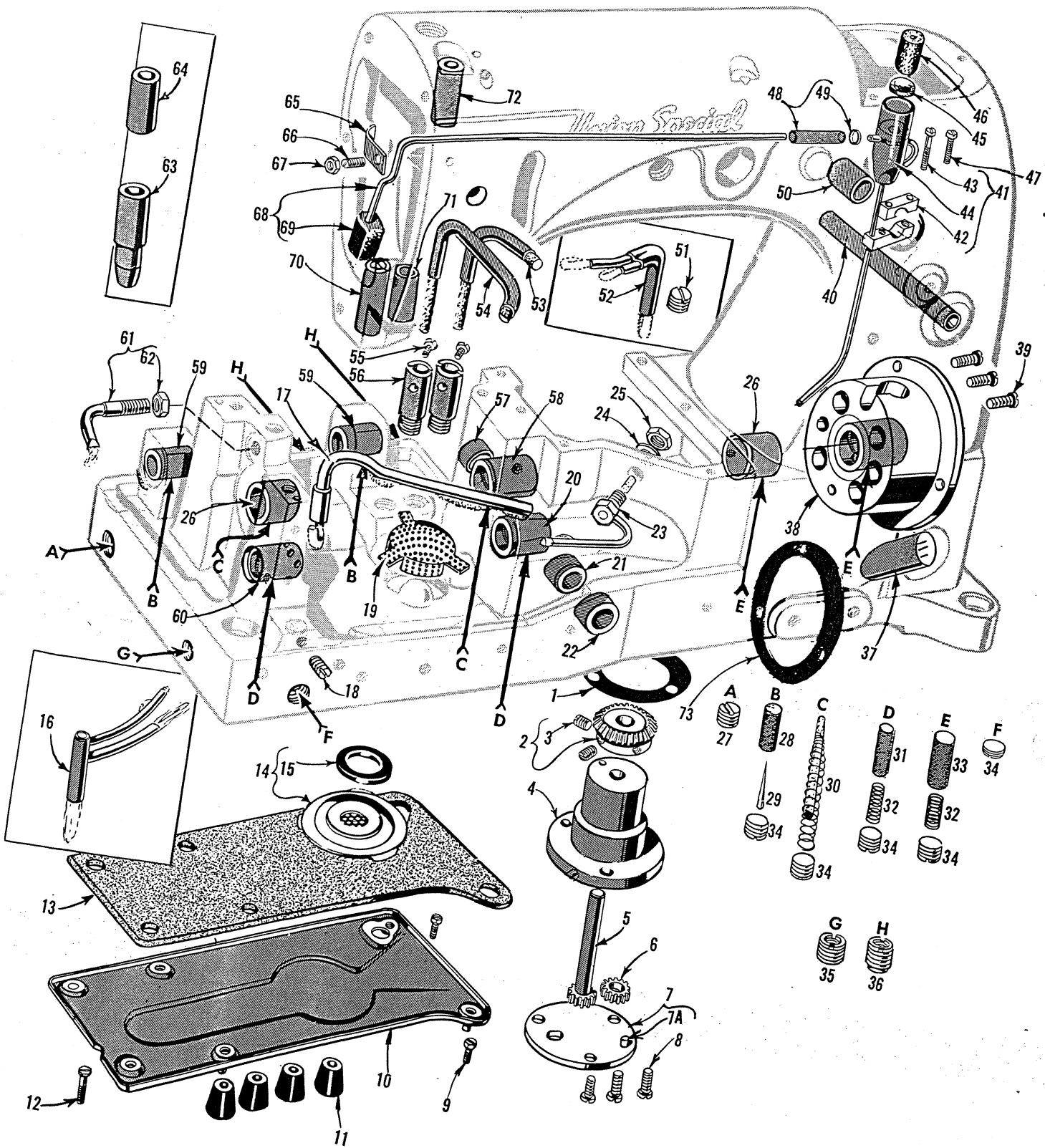
MAIN FRAME, BUSHINGS AND MISCELLANEOUS OILING PARTS
