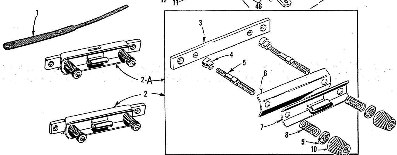
ATTACHMENTS, STRIP TENSIONS AND COLLAPSING MECHANISM
