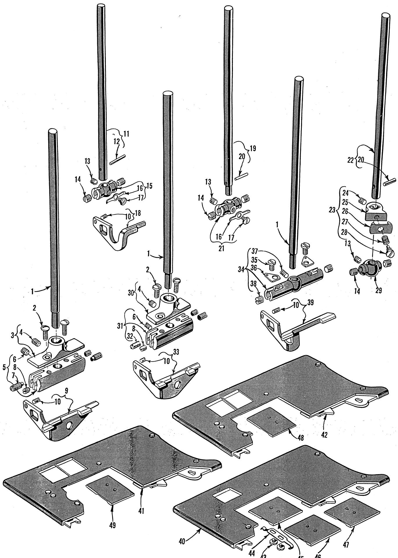
NEEDLE BARS, NEEDLE HOLDERS, NEEDLE GUARDS, CLOTH PLATES
