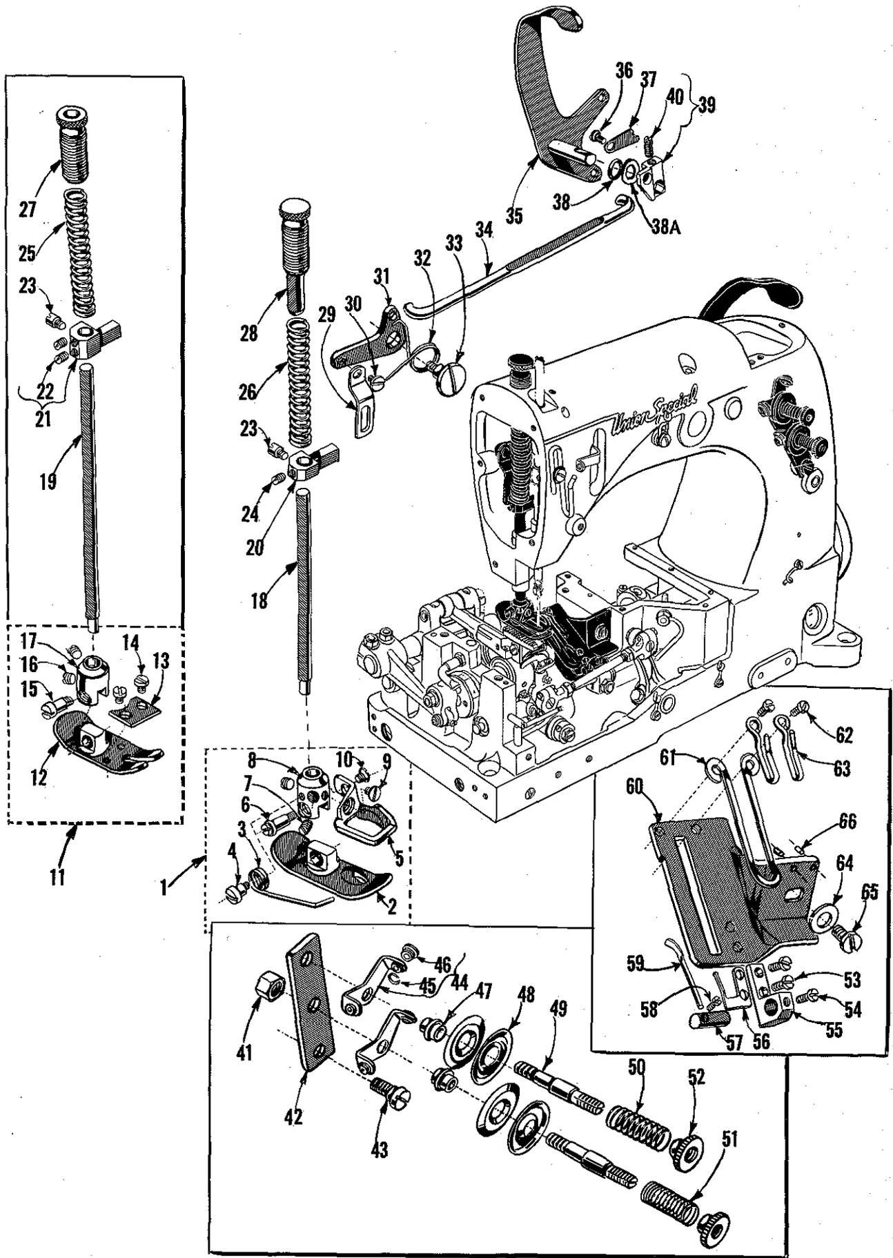
PRESSER FEET, LIFTER LEVER AND THREAD TENSION PARTS
