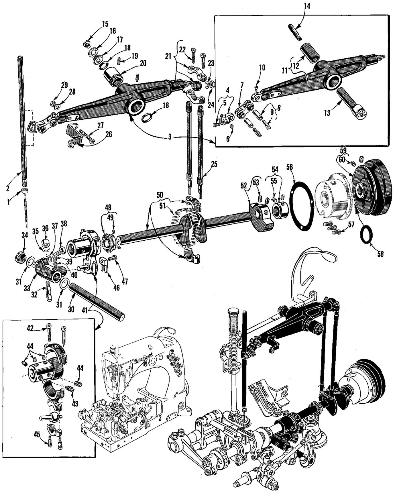
CRANKSHAFT, NEEDLE LEVER AND LOOPER DRIVING PARTS
