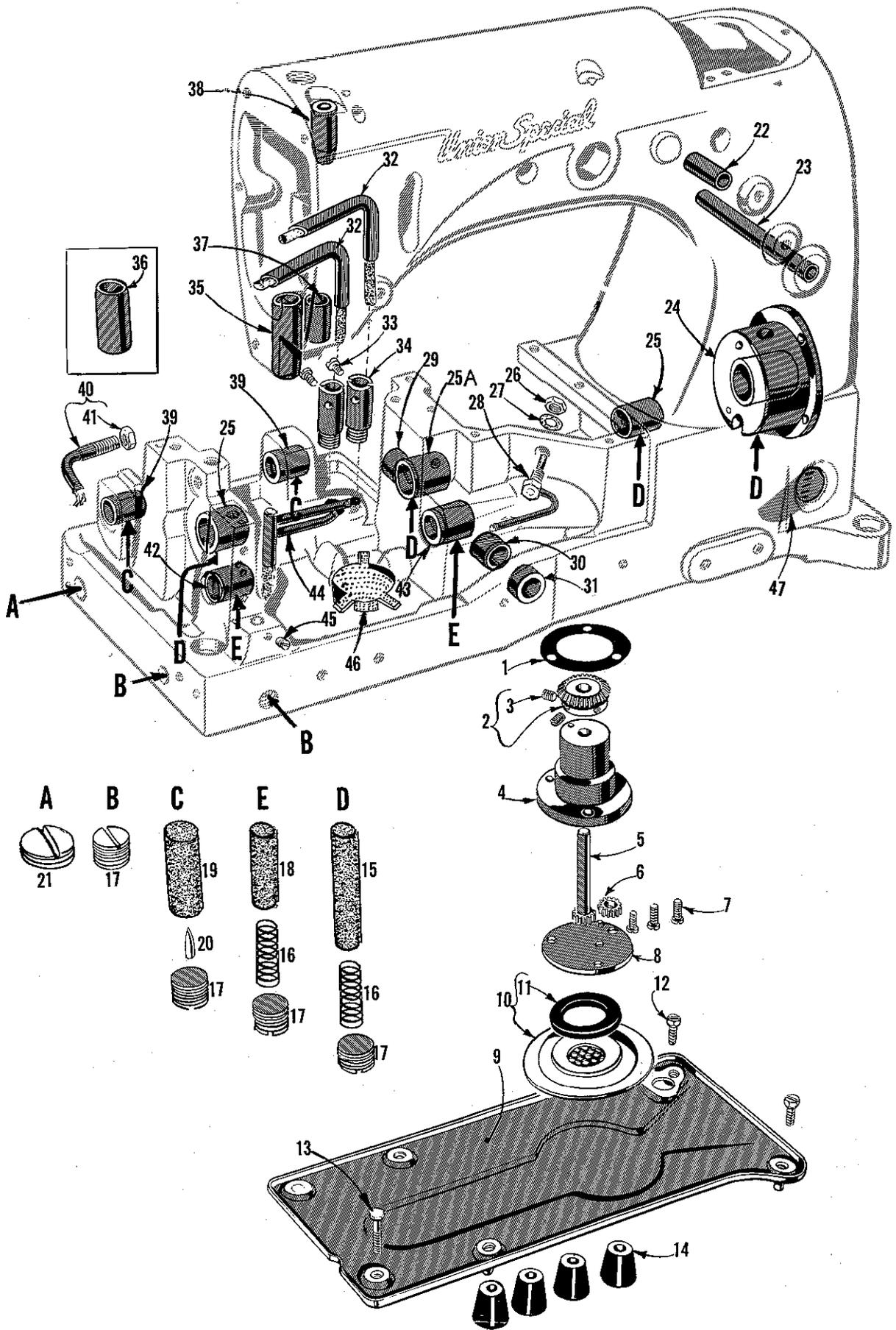
MAIN FRAME, BUSHINGS AND MISCELLANEOUS OILING PARTS
