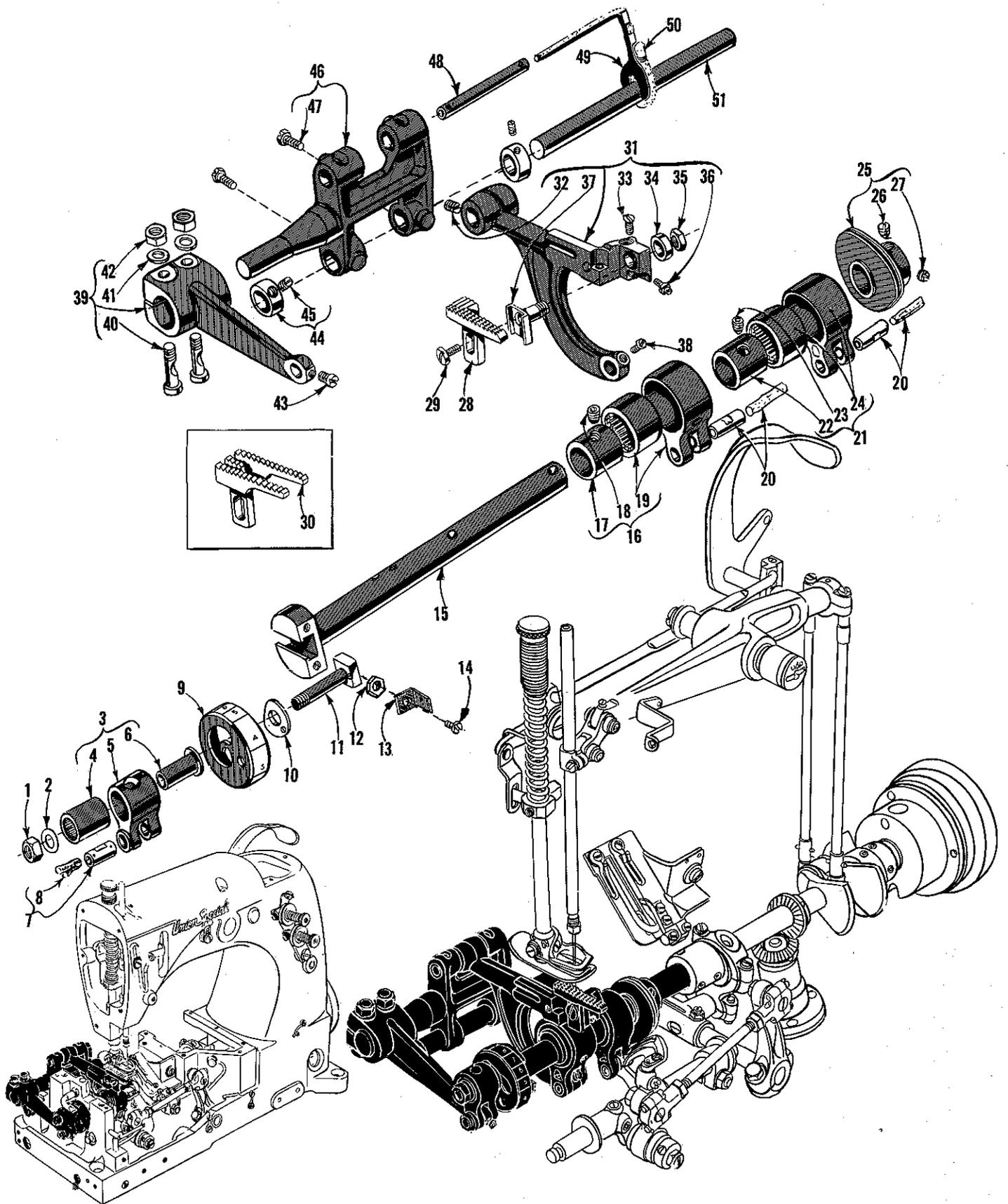
MAIN SHAFT AND FEED DRIVING PARTS
