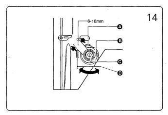
The stroke of the thread take – up spring runs from 8mm to 10mm, when sewing very thin fabrics, reduce the thread take – up spring tension and increase the thread take – up spring stroke, where as increase the thread take – up spring tension and reduce the thread take – up stroke when sewing very thick fabries.
