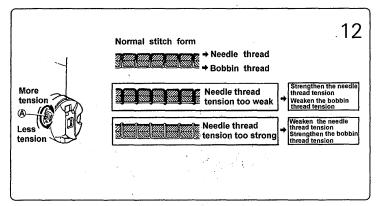
Thread tension should be determined in accordance with the stitch obtained by adjusting the tension of the bobbin thread and needle bension (Fig. 12).
