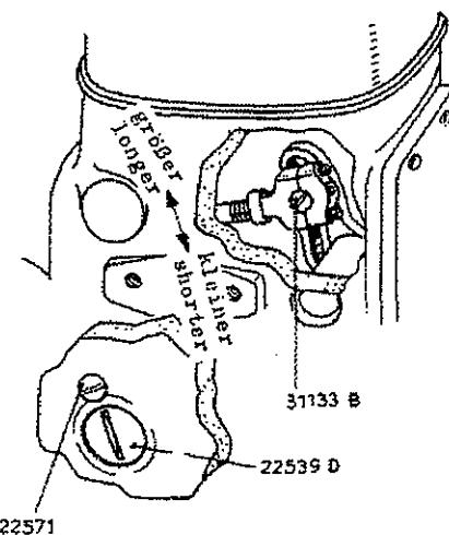
This mechanism is accessible after removing the right plug screw No. 22539 D and 22571 above the handwheel. Loosen the ball screw No. 31133 B by turning left and move it in the feeding segment. Moving downwards results in a shorter, and upwards in a longer stitch length.
