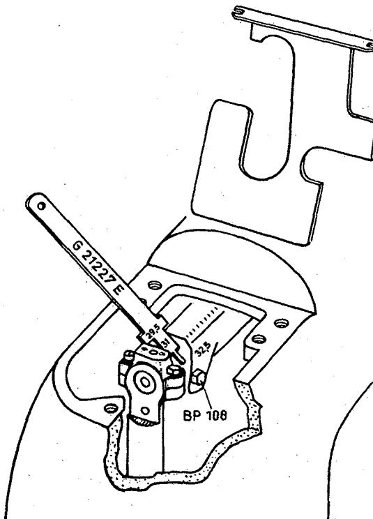
Adjusting the Stitch Length of the Non-Differential Feed Machine
