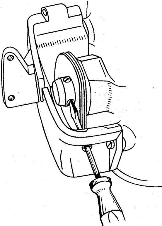
The double disc take-up must be set into the middle of cast-off plate slot. It is located at the left side of the crank shaft and is adjustable with two set screws (see sketch). When the needles move downwards and the looper begins to travel from extreme right to left, the take-up must contact the looper thread so that all slack is removed. The looper thread should cast off the high point of the take-up when the looper with its eye is at the right threaded needle.
