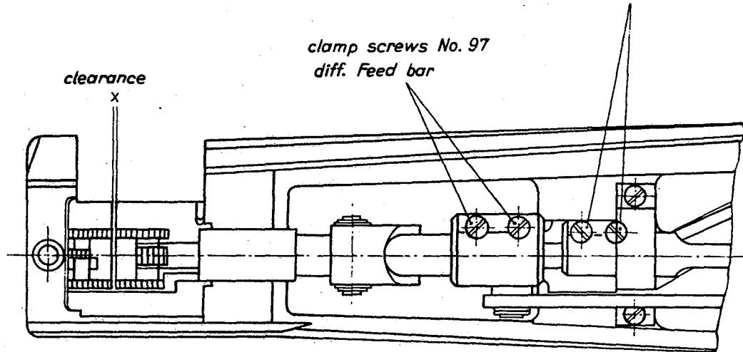
Now the feed bars are accessible and adjustable by loosening clamp screws No. 31135 B and No. 97 (see sketch). After finishing adjustment tighten clamp screws and replace cylinder arm cover with gasket and rubber sealing cord. Damaged gaskets or rubber sealing cords should be replaced by new ones.
