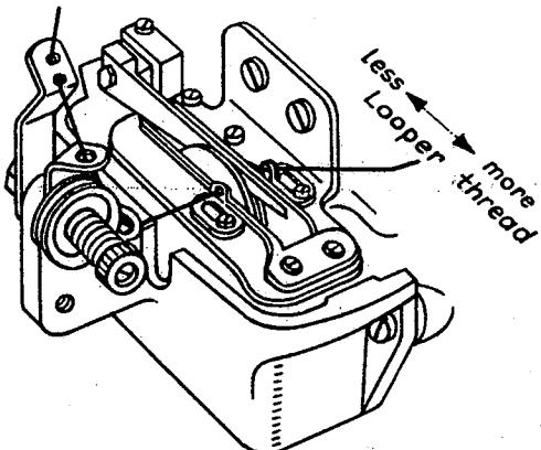
At the right and left side of the double disc take-up on the cast-off plate there are adjustable thread eyelets. These eyelets must be set as close as possible to the double disc take-up. To adjust these eyelets towards the operator results in more looper thread in the system and moving them in the opposite direction, less looper thread will be drawn.
