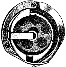
Figure G Correct Position of Hook for Re- moving Gib Screws and Gib.
